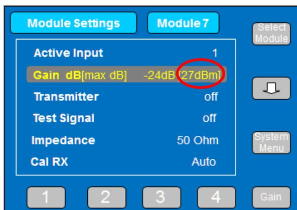
The maximum allowable input that may be applied can be toggled between dBm, dB $\mu$ V and mV.
