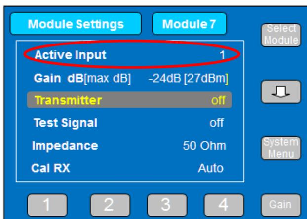
The other inputs may be selected by pressing the buttons below the icons numbered 1 to 4 on the system controller display.
