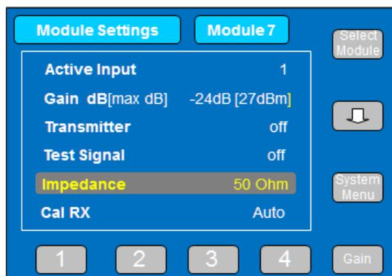
Rotate the function wheel to change the impedance. The Sentinel IIsc FOL has been optimised for ultra-wide bandwidth and wide dynamic range. As a result, the attenuators and other wideband circuits are all 50Ω, and the High Impedance buffer circuit is placed before these circuits in the Transmitter. **The gain of the system should be set to 21dB when the High Impedance mode selected**, as operation at other system gains is likely to compromise the noise and linearity performance of the system.
