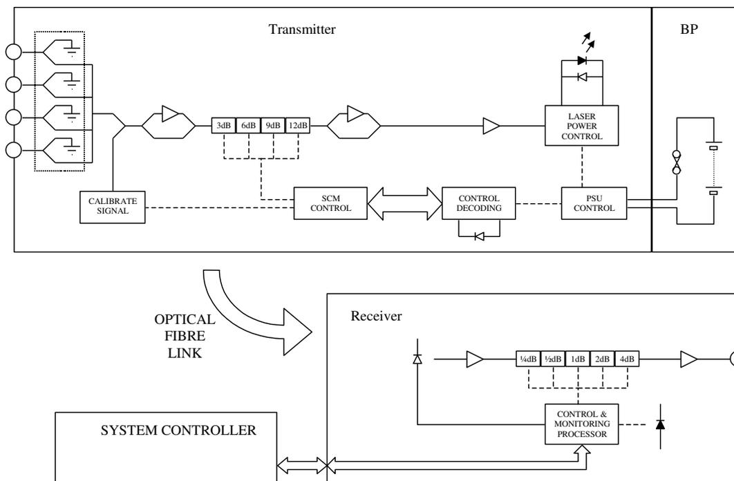
The Sentinel / Sentry IIs Sc Fibre Optic Link uses Intensity Modulation (IM) for the transmission of analogue data from the Transmitter to the Receiver. This scheme offers unparalleled levels of bandwidth and dynamic range when compared to alternative modulation methods.
