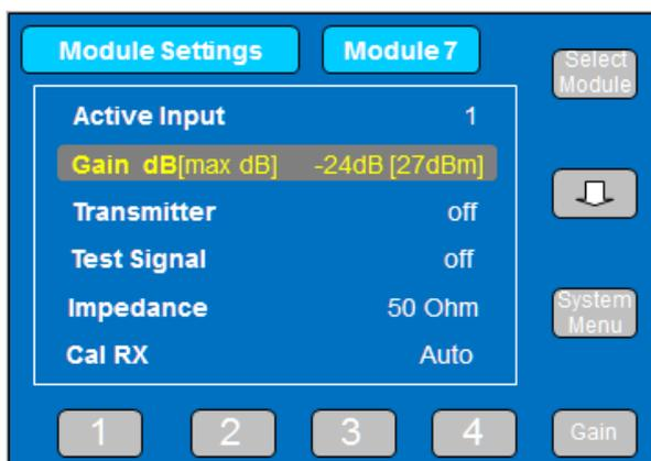
This can be achieved by, either stepping through the selections using the down arrow, or using the gain shortcut button, this is below the “Gain” icon.
