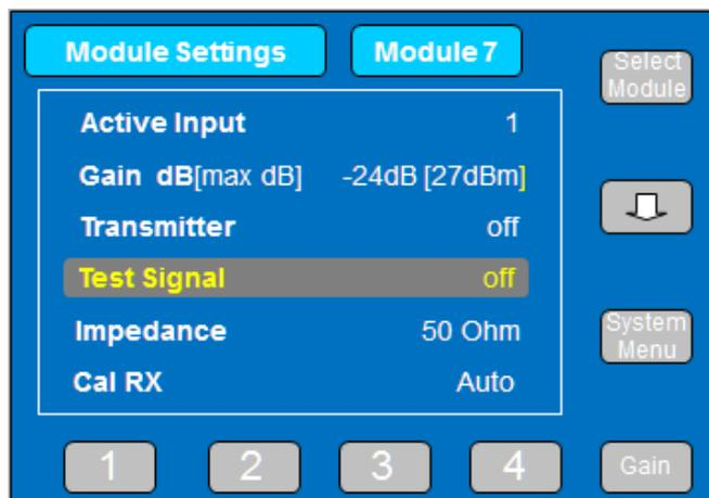
Rotate the function wheel to enable/disable the test signal.
