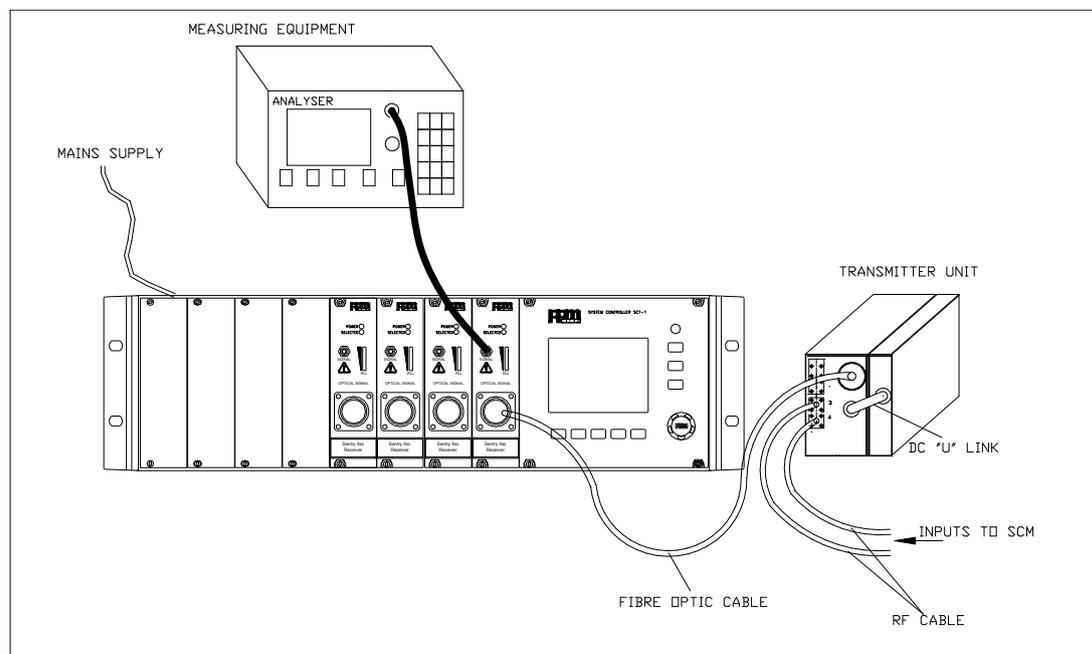
Once all the connections are made to the units, the System Controller can be switched on. All functions of the Transmitter and Receiver are controlled through the System Controller unit.
