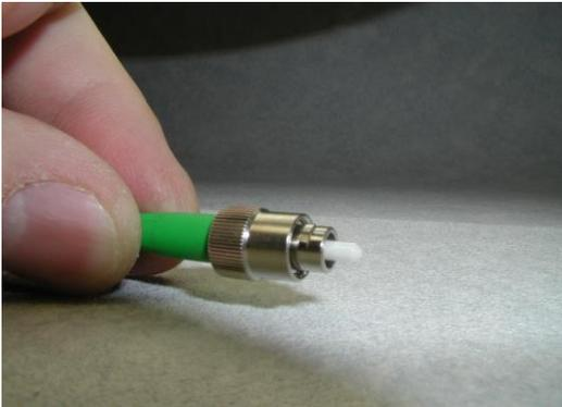
2. Insert Connector ferrule into connector feed through.
