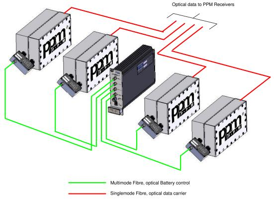
Layout for optically controlled battery switches when used in conjunction with PPM shielded batteries. For illustrative purposes only; control module normally resides with receivers in a suitable PPM 19" rack case)
