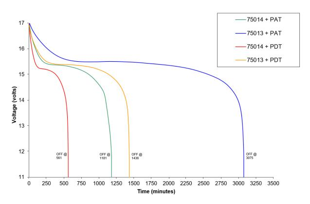
The data above shows the discharge performance characteristics for all variants of the Power Sleeve when running a standard *point2point* AC or DC link, including the effect of using the optically controlled battery switch, which increases the speed at which the battery discharges.
