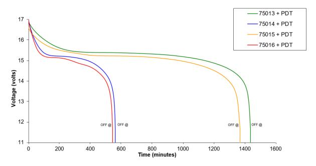
Typical discharge time for 9 Ah & 3.6 Ah power sleeve options when powering either a DC or AC link
