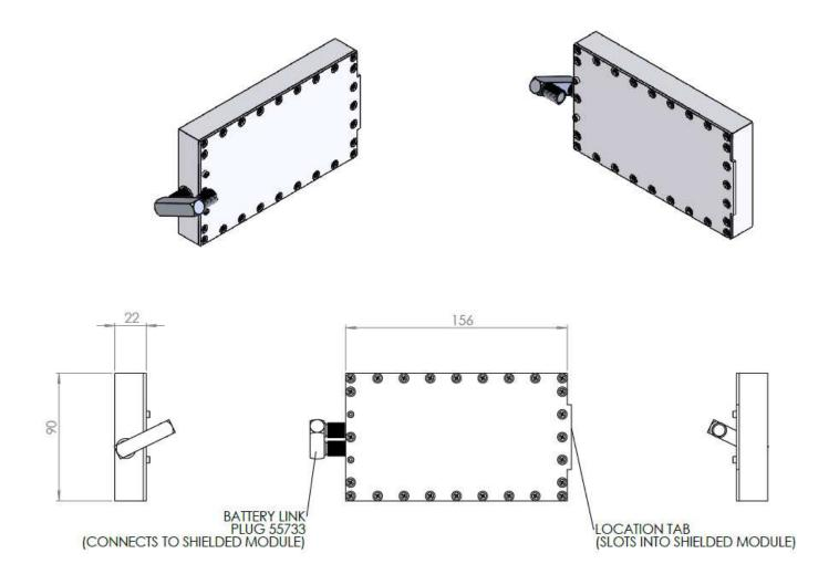
Shielded high capacity battery pack (3.6Ah) 73512 (includes battery link plug 55733)
