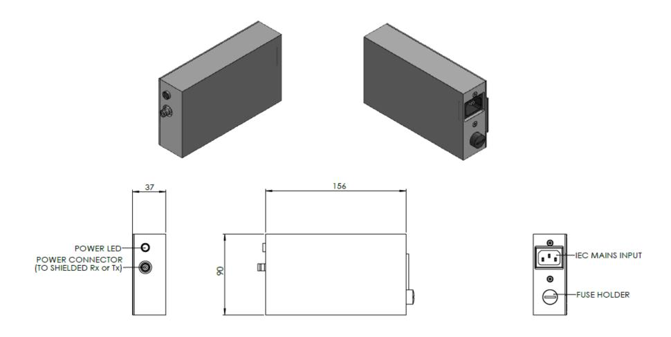
Shielded standard battery pack (2.0Ah) 73511 (includes battery link plug 55733)
