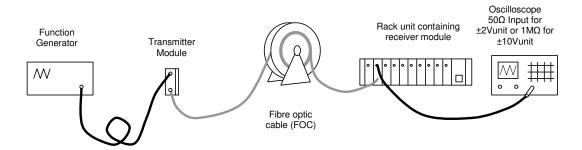
The sequence in which the equipment is initially set up to make a measurement is not critical, though it is recommended that the fibre optic cable is attached to both transmitter module and receiver module before the transmitter module is powered up. This way, there is no optical hazard presented by laser light propagating through a free end of the fibre.
